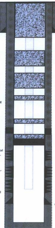
Plug #6:Surface shoe, 331'- surface. Pumped 39sx of Class G cmt & spot balanced plug inside casing.
