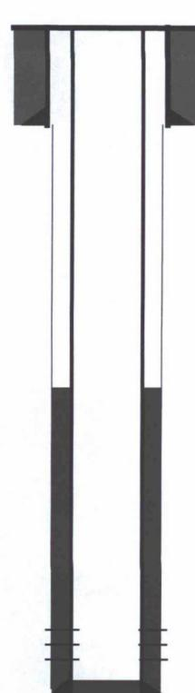
8 5/8" J-55 24# casing @ 167'. Cemented with 130 sks Type III w/ 2% gel. Hole size 12-1/4"
