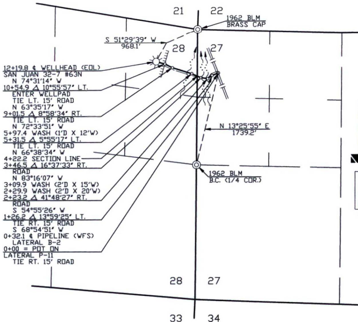
NOTE: BEARINGS ARE BASED ON A GRID BEARING. ALONG THE EAST LINE OF THE NE 1/4 OF SECTION 28, T-32-N, R-7-W, NMPM BEARS: S 0°31'24" W
