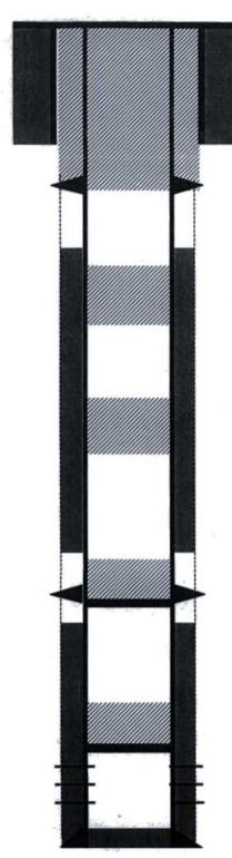
8 5/8" J-55 24# casing @ 166'. Cemented with 100 sks Class A w/ 2% gel. Circulated cement to surface
