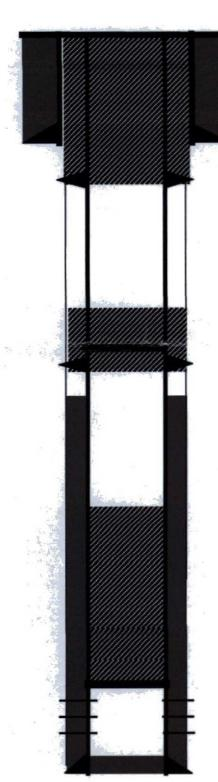
8 5/8" J-55 24# casing @ 167'. Cemented with 130 sks Type III w/ 2% gel. Hole size 12-1/4"
