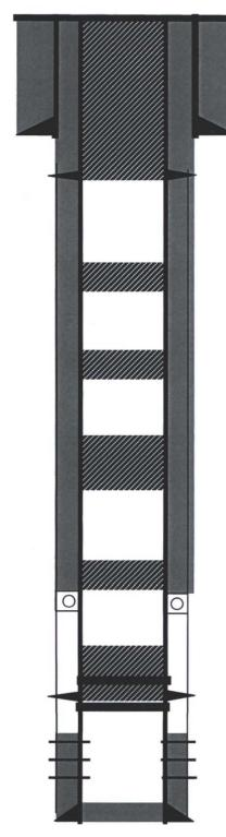
$8\ 5/8"$  J-55 24# casing @ 200'. Cemented with 135 sks Class B w/ 2% gel. Circulated cement to surface
