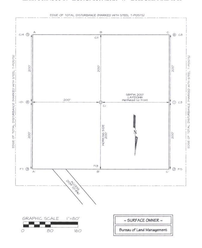
Steel T-Posts have been set to define the Edge of Disturbance limits which are 50' offset from the edge of the staked wellpad.
