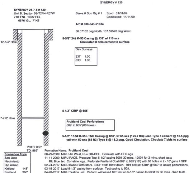
04-20-2017 MIRU Testing unit. Perform witnessed MIT test on 5-1/2" casing to 596# for 30 mins, chart tests. Performed witness bradenhead test. Well Secure.
