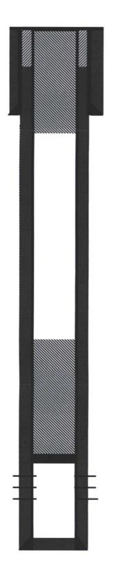
7" 20# ST & C casing @ 94'. Cemented w/ 35 sks, 41 cu.ft.
