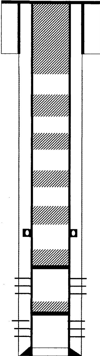
8 5/8" J-55 24# casing @ 200'. Cemented with 135 sks Class B w/ 2% CaCl2. Circulated cement to surface.
