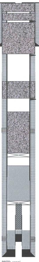
PBTD: 2000' TD: 6330' Perforate @ 60' Sept 2017-Plug #3: 60' - 0' Class B cement, 148 sxs
