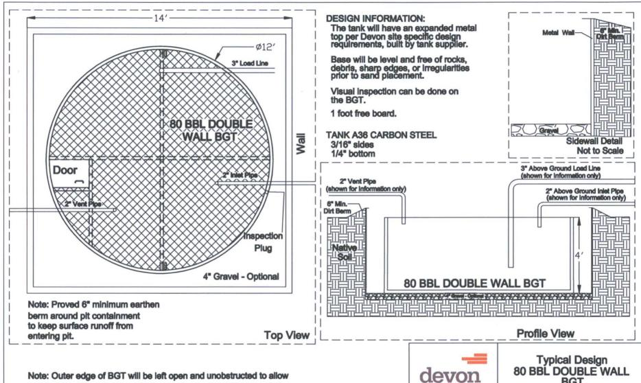
for visual inspection of secondary containment for evidence of leaks.
