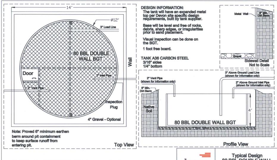
Note: Outer edge of BGT will be left open and unobstructed to allow for visual inspection of secondary containment for evidence of leaks.
