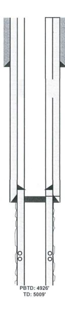
Hole Size: 12-1/4" Surface Csg: 10-3/4" Hole Size: 8-3/4' Int Csg: 7" Prod Csg: 5" 15#
