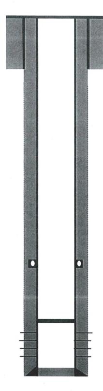
8-5/8" J-55 24# casing @ 221'. Cemented with 150 sks, 177 cf Class B w/ 2% CaCl2. Circulated 3 bbl cement to surface. Hole size: 12-1/4
