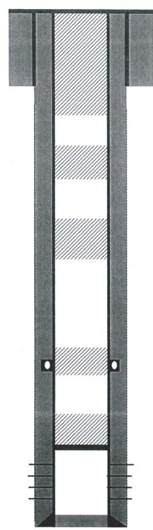
8-5/8" J-55 24# casing @ 221'. Cemented with 150 sks, 177 cf Class B w/ 2% CaCl2. Circulated 3 bbl cement to surface. Hole size: 12-1/4
