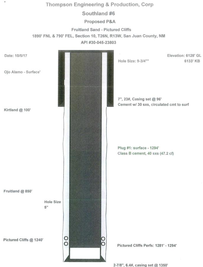
PBTD: 1313' TD: 1350' 2-7/8", 6.4#, casing set @ 1350 Cement w/ 140 sx Circulated cement to surface
