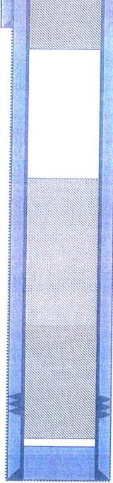
TD 1230' PBTD 1185' Plug #1: 1161' - 808' Class G cement, 36 sxs (30% excess long plug)
