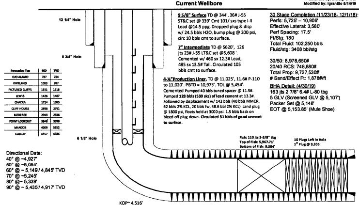
Perf'd @ 5725'-10906', 0.35" & .42" diameter w/ 1044 total holes. Frac'd @ 5725'-10925' w/ 30 stages of 30/50 sand. PBTD: 9,305 TD: 11,025 MD TVD: 4,915.07
