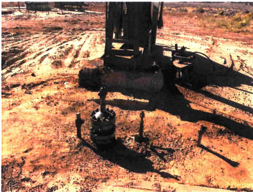
Figure 4. Wellhead and soil staining around well looking southerly.
