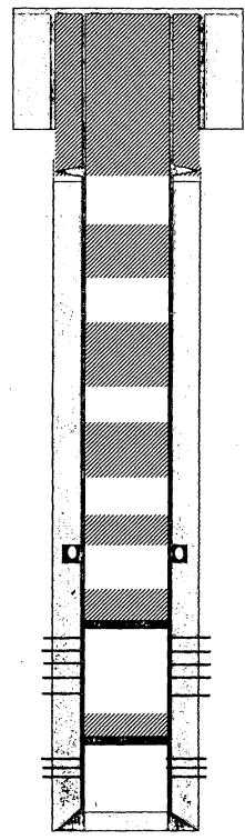
8-5/8" J-55 24# casing @ 222'. Cemented with 125 sks, 147 cf Class B w/ 2% CaCl2. Cement circulated to surface. Hole size: 12-1/4
