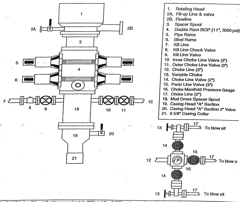
A 12-1/4" hole will be drilled to approximately 220' and the 9-5/8" surface casing will be run and cemented. The Casing Head "A" Section will be screwed onto the 9-5/8" surface casing stub. The BOP will be installed on the Casing Head "A" Section. /\*
