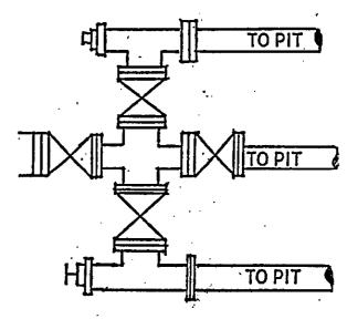
Kill line will be minimum 2" diameter and have 2 valves, one of which shall be a minimum 2" check valve.
