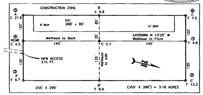
RESERVE PYT DIKE: TO BE 8' ABOVE DEEP SIDE (OVERFLOW - 3' WIDE AND 1' ABOVE SHALLOW SIDE). BLOW PIT: OVERFLOW PIPE HALFWAY BETWEEN TOP AND BOTTOM AND TO EXTEND OVER PLASTIC LINER AND INTO BLOW PIT.
