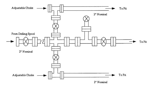
Choke manifold installed from surface to TD
