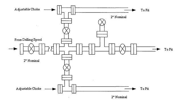
Choke manifold installed from surface to TD
