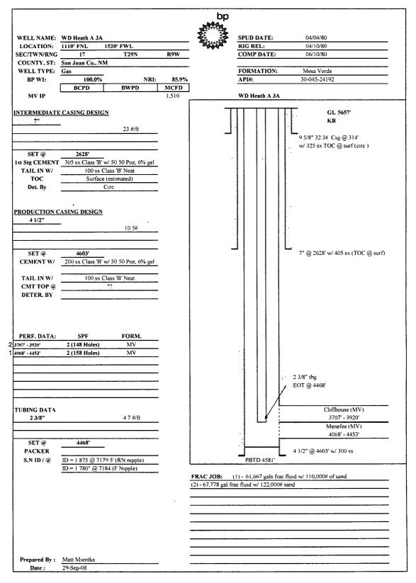
Figure 1: Well Schematic for the W D Heath A 3A
