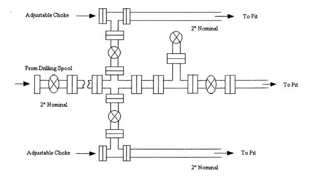
Choke manifold installed from surface to TD
