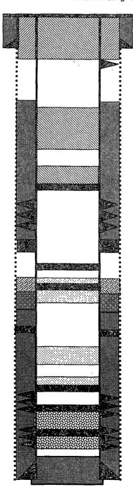
8.625" 24#, J-55 Casing set @ 213' Cement with 165 cf, circ to surface.
