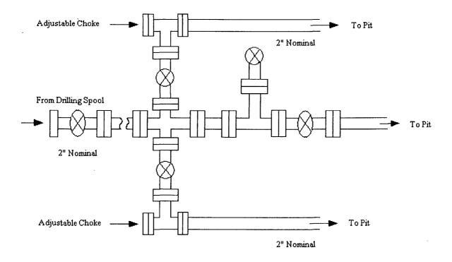
Choke manifold installed from surface to TD
