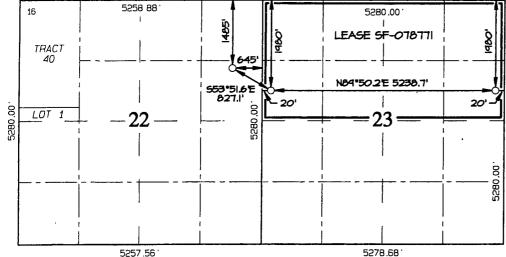
THE HORIZONTAL LATERAL REPRESENTED ON THIS PLAT CORRESPONDS TO THE BLACK SEGMENT WHICH VARIES IN THE ELEVATION FROM 6891.0' AT THE POINT-OF-ENTRY TO 6749.0' AT THE END-OF-LATERAL.
