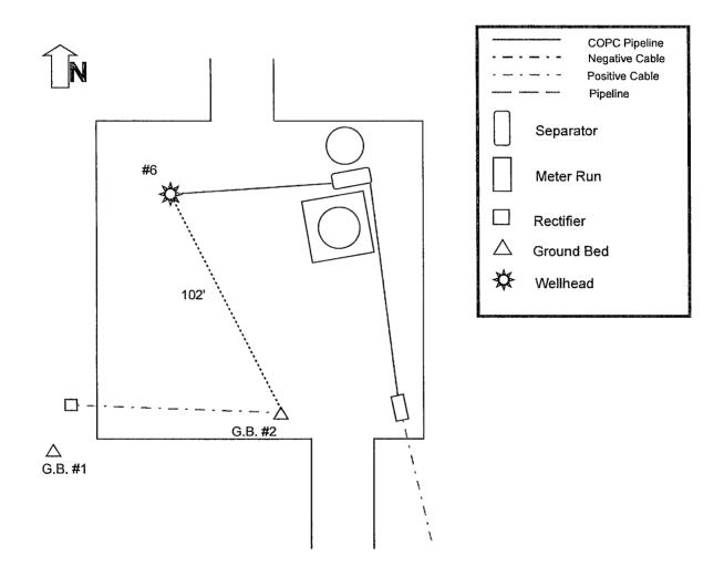
Drill new ground bed approximately 102' South East of #6 wellhead at staked location. Run new positive cable from existing rectifier mounted on FEUS meter pole #58715926 to new ground bed #2 at length listed below.
