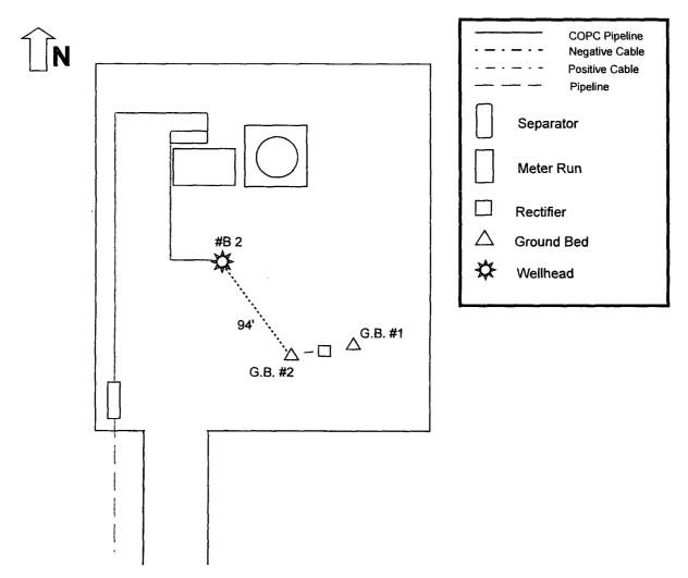
Drill new ground bed approximately 94' South East of #B 2 wellhead at staked location. Run new positive cable from existing rectifier to new ground bed at length listed below.
