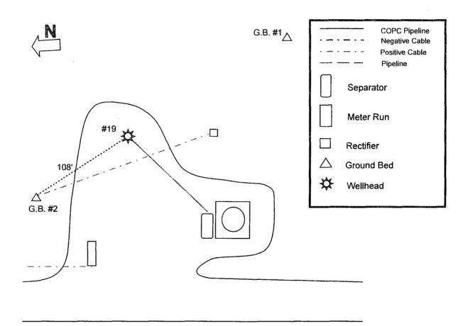
Drill new ground bed approximately 108' North West of #19 wellhead at staked location. Run new positive cable from existing rectifier to new ground bed #2 at length listed below.
