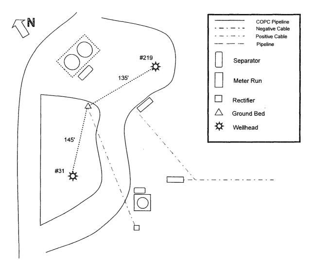
Drill new ground bed approximately 135' West of #219 wellhead at staked location. Run new positive cable from existing rectifier to new ground bed at length listed below.
