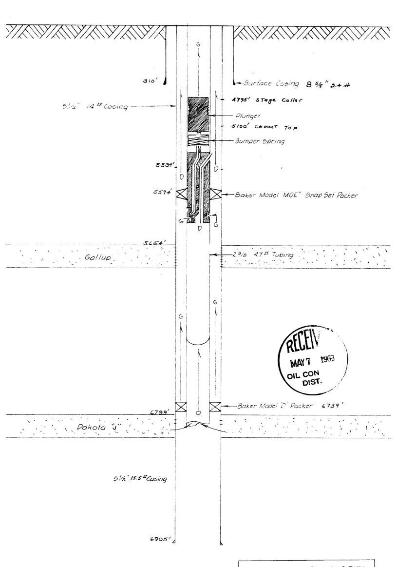
SCHEMATIC DIAGRAM of DUAL COMPLETION of NE. HAYNES
