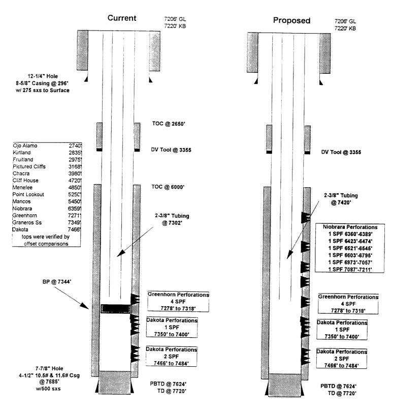
The Dakota is temporarily abandoned under a drillable bridge plug. The Greenhorn is on production test.
