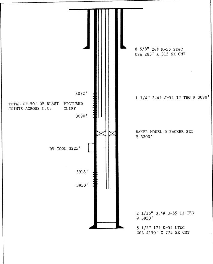
CENTRALIZERS RUN EVERY OTHER JOINT FROM TD TO 3735' AND FROM DV TOOL TO 2850'.
