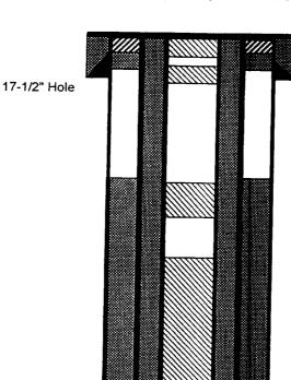
4-1/2" TOC at Surface, circulated 5 sxs cement; 8-5/8" TOC Unknown, 50 sxs(127') pumped into BH annulus, then took 8 bbls water to load (96' down
