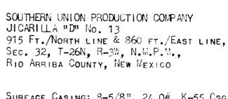
SURFACE CASING: 8-5/8", 24.0#, K-55 Csg. SET AT 234 FT. R.K.B. CEMENTED TO SURFACE W/150 SACKS CEMENT.
