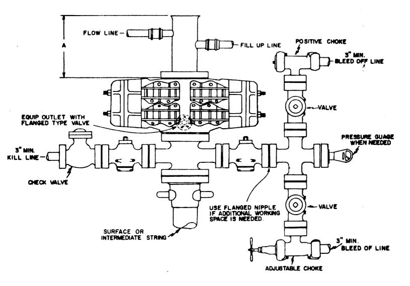
NOTE: BLOWOUT PREVENTER MUST HAVE DOUBLE RAMS; ONE BLIND 8 ONE PIPE RAM OR THE EQUIPMENT MUST CONSIST OF TWO BLOWOUT PREVENTERS, ONE EQUIPPED WITH BLIND RAMS 8 THE OTHER WITH PIPE RAMS. ALWAYS PLACE THE BLIND RAMS IN THE TOP PREVENTER.
