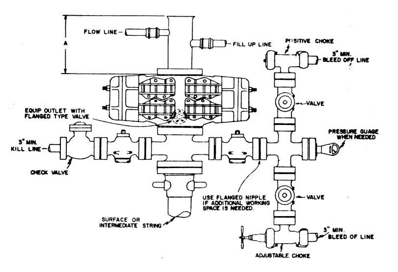
NOTE: BLOWOUT PREVENTER MUST HAVE DOUBLE RAMS; ONE BLIND & ONE PIPE RAM OR THE EQUIPMENT MUST CONSIST OF TWO BLOWOUT PREVENTERS. ONE EQUIPPED WITH BLIND RAMS & THE OTHER WITH PIPE RAMS.
