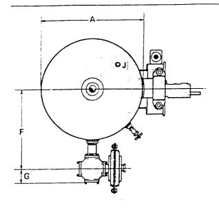
For measurement of liquid produced from individual wells, individual zones or individual leases under a common royalty account. Also, a LIQUA-METER unit may be used in conjunction with a test separator or treater to determine the production of individual wells or zones without interrupting the production of other wells which continue to flow through the common production facilities. A pneumatic totalizer records the number of dumps of the meter and is convertible to barrels run during the test.
