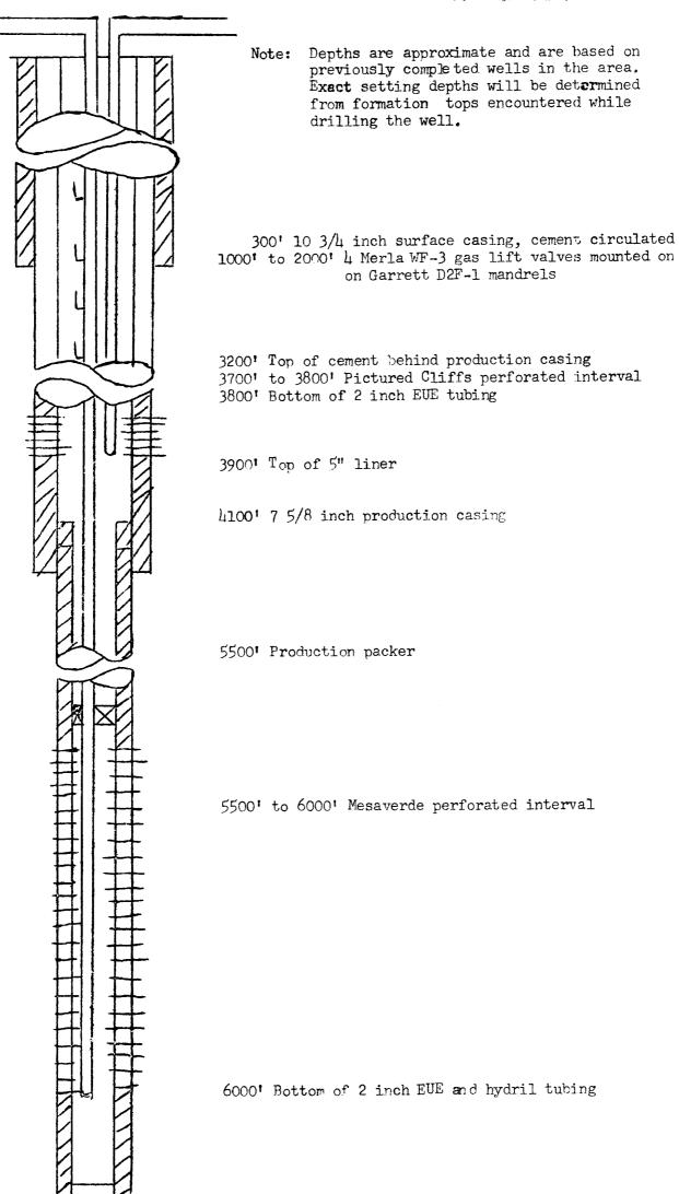
6300' Total depth, Bottom of 5 inch liner, cement
