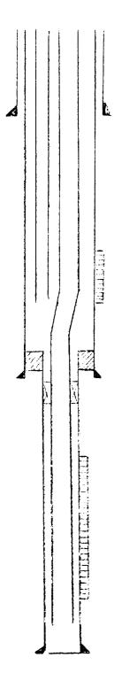
9-5/8", 32.30#, H-40 casing set at 221'. Cemented with 125 sacks (148 cu.ft.)
