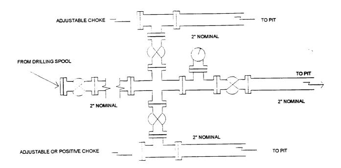
Minimum choke manifold installation from surface to Total Depth. 2" minimum, 3000psi working pressure equipment with two chokes.
