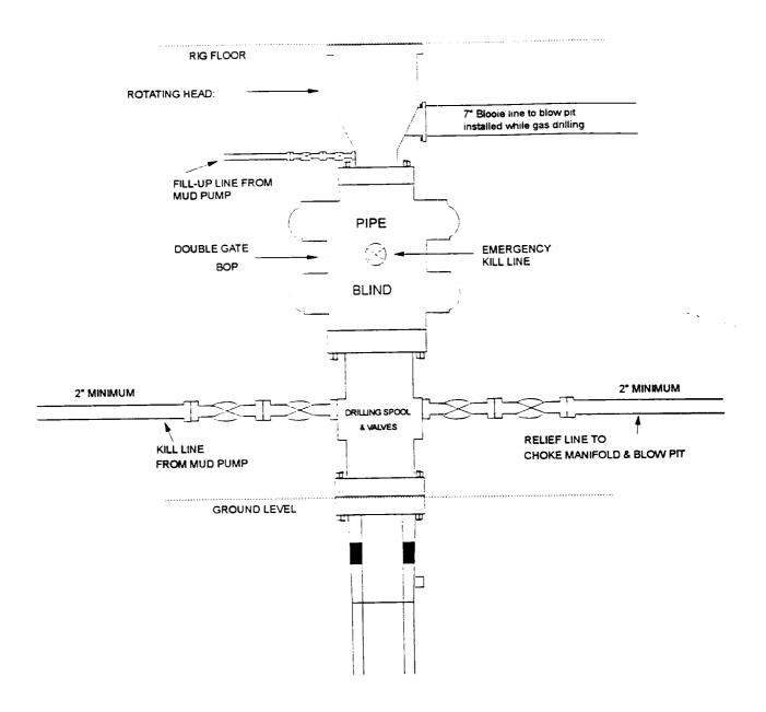
11" Bore, 3,000psi minimum working pressure double gate BOP to be equipped with blind and pipe rams. A Schaffer Type 50 or equivalent rotating head to be installed on the top of the BOP. All equipment is 3,000psi working pressure/or greater.
