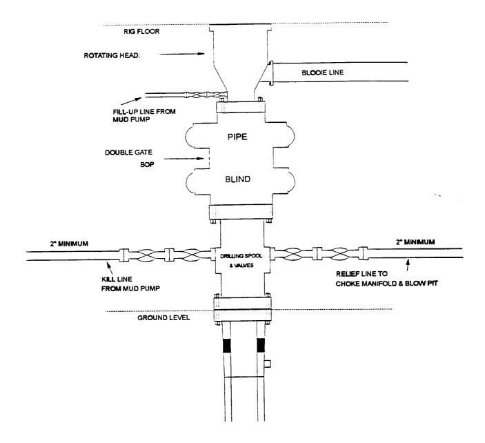
Minimum BOP installation for Completion operations. 7 1/16" Bore (6" Nominal), 3,000psi minimum working pressure double gate BOP to be equipped with blind and pipe rams.
