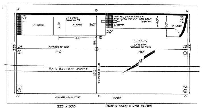
Reserve Pit Dike: to be 8' above Deep side (overflow - 3' wide and 1' above shallow side). Blow Pit: overflow pipe halfway between top and bottom and to extend over plastic liner and into blow pi
