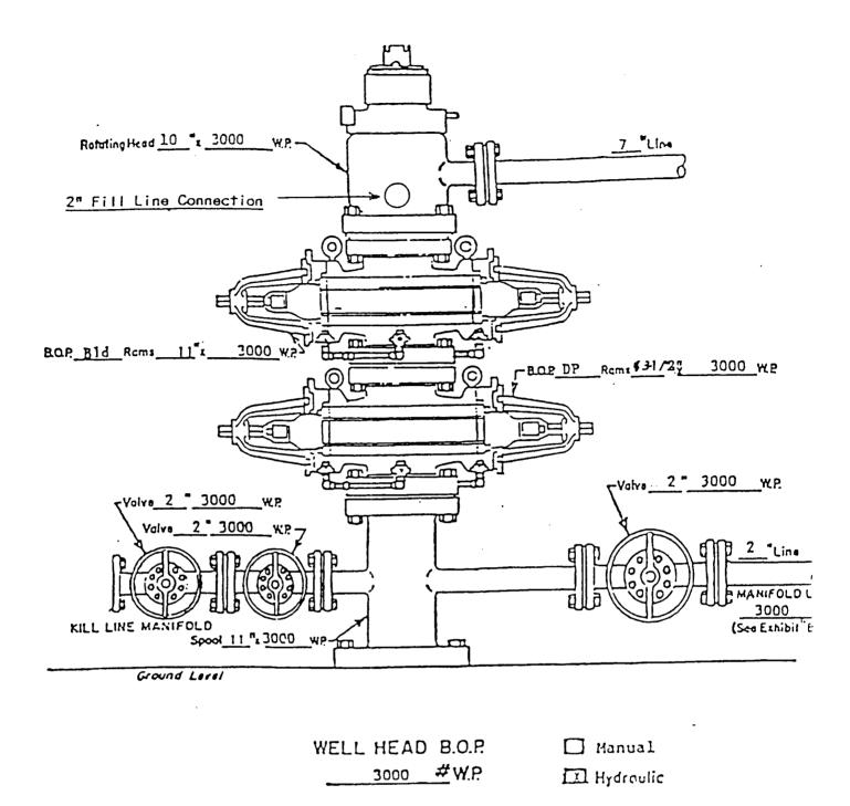
NOTE: Although 3000 psi 80P equipment will be used, equipment determination and line sizing are based on the requirements for 2000 psi BOP equipment due to the known drilling and reservoir conditions.
