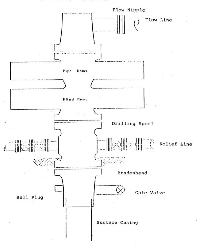
800 Series 900 Double Gate BOP, rated at 3000 psi Working Pressure
