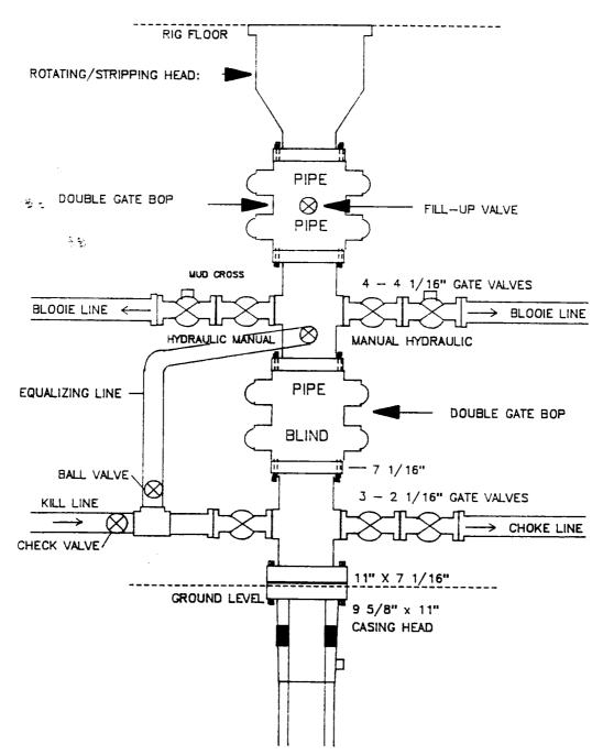
Minimum BOP installation for a typical open—hole Fruitland Coal well from intermediate TD to TD. 7 1/16" Bore (6" Nominal), 2000psi working pressure/ or greater double stack double gate BOP equipped with three pipe and one blind ram.
