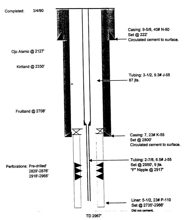
Workover History: 7/98 - Pulled tbg, fished for liner, jarred loose, pressure tested & replaced liner & tbg.
